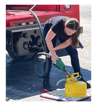
The smart polymer solidifies hydrocarbons, trapping the pollutants inside the spill pad.
